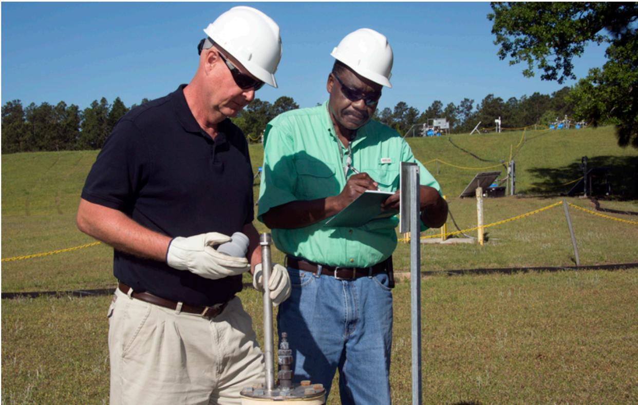
Caption: John Bradley, Design Authority Engineer (left) and Joao Cardoso-Neto, Upper Three Runs Project Manager, both with the SRNS Area Cleanup Projects organization, inspect a BaroBall™ unit. This remediation technology operates completely on natural changes in barometric pressure to pump chemical contaminants from the subsurface.
